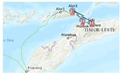
**Figure 2.** Current Broadband Infrastructure Alor – Husbuk – Dare Via Microwave *Source:* developed by the authors.
